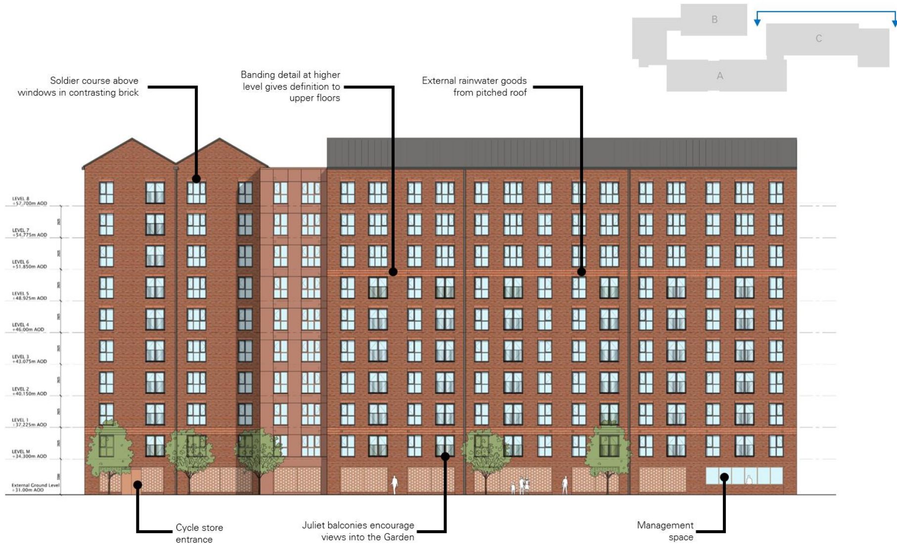
Building C: Elevation to Garden
